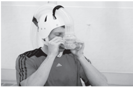
Picture 2: helmet with the mounted respiratory analyzer
